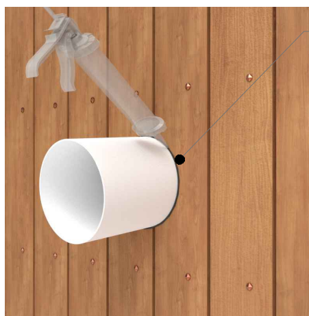
Continuous weather seal around pipe
