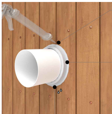
No sealant to drain
